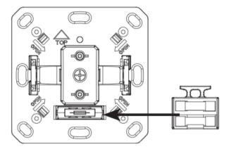
NOTE: The micro-fuse deals with a backup for the equipment that is specifically designed to this radio-controlled wireless dimmer/ switch. Please use only this fuse type. This micro- fuse should protect this radio-controlled wireless dimmer/ switch from overload and short circuits. When using another fuse component there is a danger that the device can be destroyed. A spare fuse is provided in the fuse holder.
